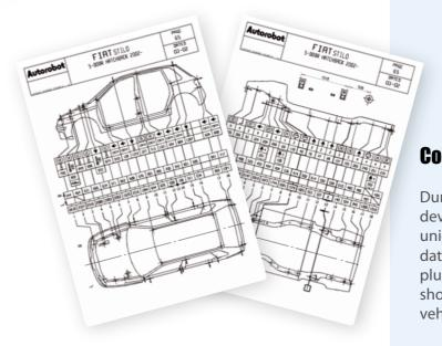
The measurements are taken between the measuring targets. The results are entered in the computer into the measuring software that saves the measured values in the database and shows the differences compared to car manufacture's values. The saved measuring values can be printed in separate reports before of after the chassis and upper body repair.
