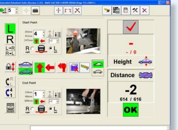
Measuring software uses large numbers, so the measuring process can easily be followed even at a distance. Measuring window indicates both reference value and actual value plus the existing difference. Results outside the accepted tolerance appear with a clear red arrow.
